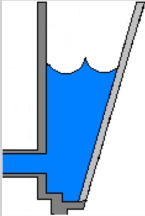
**GFS Lateral Flow Thickeners** are the most effective method for removing excess liquids from all biological sludges and many industrial sludges. Gravity Flow Systems Southwest, Inc. Lateral Flow™ Thickeners require no direct energy or power input. Unwanted liquids are separated by taking advantage of natural phenomena.
