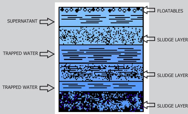
Allow sanitary sewer or many industrial waste sludges to stand, and the influences of specific gravity and fluid mechanics cause the components to separate. Floatables rise to the surface, while heavy elements sink to the tank floor.
